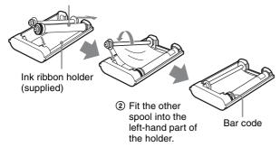
Remove any slack from the ink ribbon. If the ribbon is left slack, it may be crumpled and damaged when inserted.
